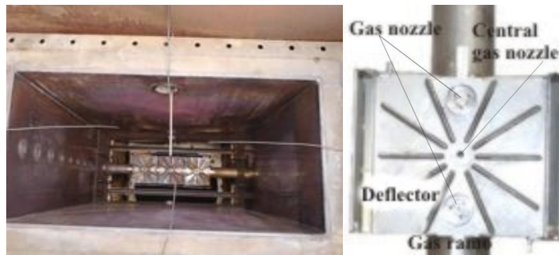
Fig. 1 The 2xST 18 Powerplant afterburner equivalent, on natural gas, mounted on the test bench at INCDT COMOTI (left) and afterburner module structure (right) [5, 7]
