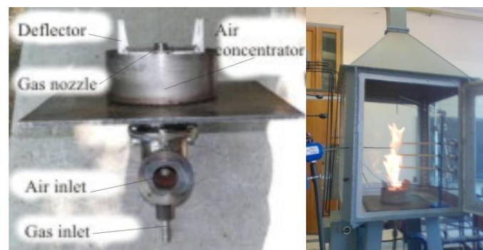
Fig. 2 Single module afterburner (left), tested on natural gas with air at UPB (right)
