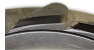
Fig. 8 The abrasion of the compressor stator within turboengine using supercritical CO 2
